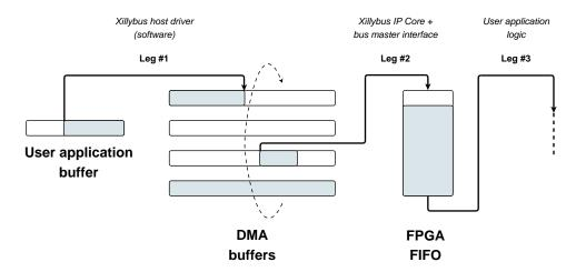
As before, the data flows from the host to the FPGA in three legs, as detailed next.
