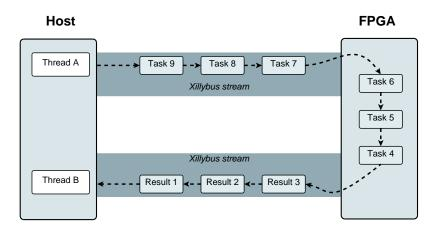
The acceleration of sqrt() is a relatively simple example, but it covers much of the challenge in utilizing coprocessing techniques. Almost always, large parts of the computer program needs to be rewritten so that the everything is driven by the pipelined data flow.
