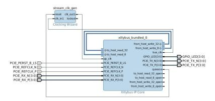
On Xillinux targets, "Open Block Design" opens the Zynq processor's environment – this block design *should not be modified* in tasks related to Xillybus. Rather, the block marked "blockdesign" should be opened (with a double-click), which displays the following block diagram:
