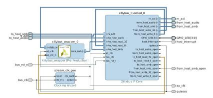
The connection between ap\_rst\_n and to\_host\_read\_32\_open holds the logic in xilly-bus\_wrapper block reset unless the xillybus\_read\_32 device file is opened on the host (to\_host\_read\_32\_open is logic '0' when the file isn't opened, and the reset input is active low). Assuming that the software running on the host opens this device file before attempting to communicate with this block, this ensures a consistent response from the logic each time the software is run.
