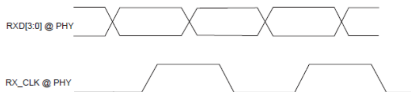
Figure 13. RGMII physical chip generated RX_CLK signal and RXD (data), with internal delay enabled. With the internal delay both signals are center-aligned [5].
